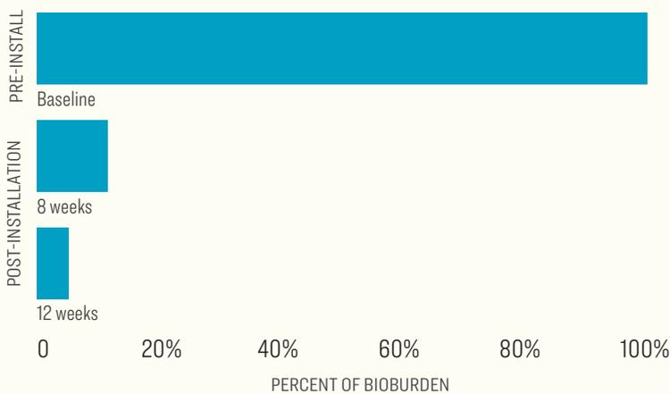
Figure 3: Results of Vyv antimicrobial lighting in an office environment.
