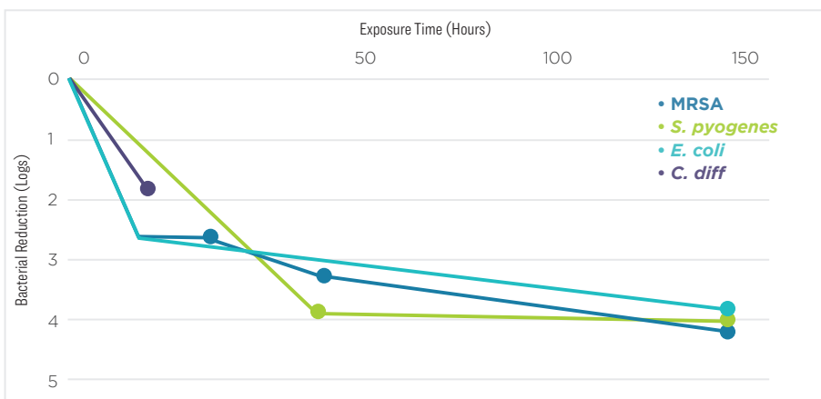
Figure 1. Bacterial reductions with increasing absolute dosages of Antimicrobial White Light. Source: NYSDOH, 2012
