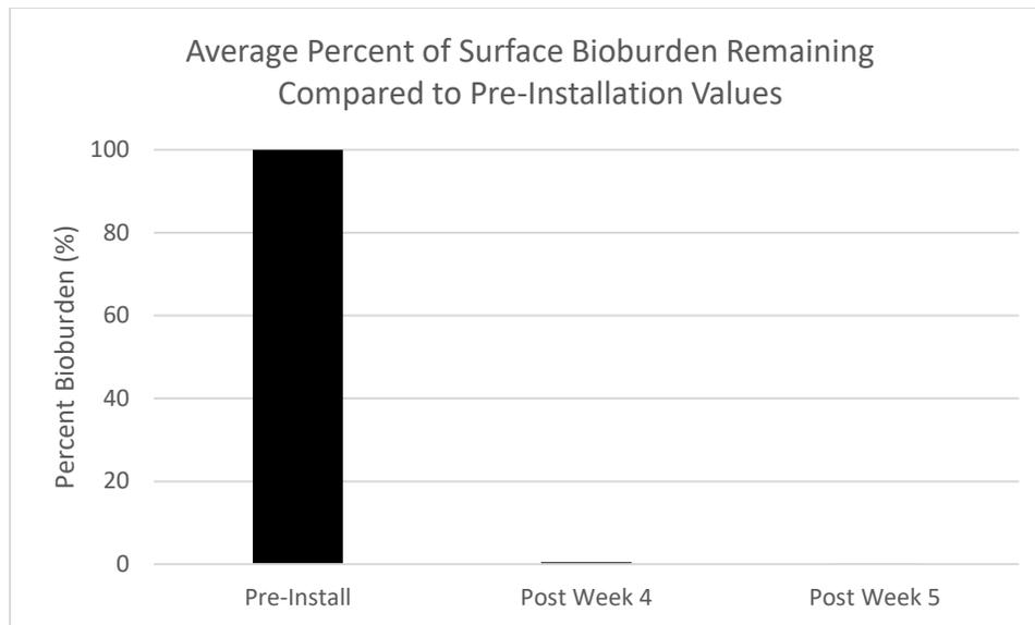
Figure 3. Comparison of the post-installation colony count data to baseline values. The baseline counts were used as 100% of the total and the percent of bioburden remaining on surfaces compared to that baseline value was calculated for each post-installation time point.
