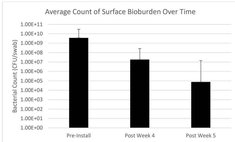
Figure 2. Geometric mean surface bioburden across all 3 sites before and after installation of Vital Vio’s antimicrobial light fixture. Error bars are indicative of the standard errors at each time point.
